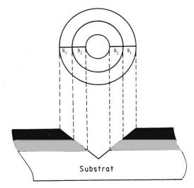
Fig. 1: Drilled hole of a two-layer coating shown in cross section and observed with microscope  $(s_1 / s_2 = Measuring distance for layers 1 / 2)$
