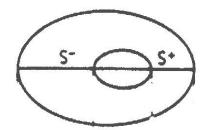
Fig. 4: View through microscope: specimen not drilled perpendicularly (s<sup>-</sup>/s<sup>+</sup> = measuring distance)
