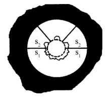
Fig. 3: View through microscope onto drilled cut out with crumbled edges  $(s_1 / s_2 = measuring distances)$
