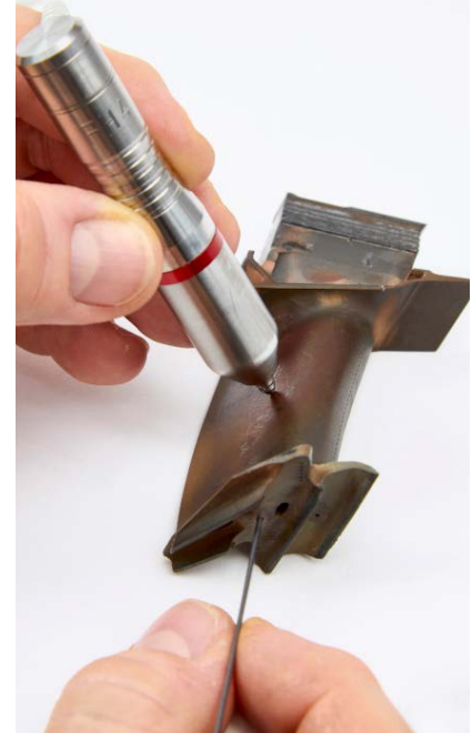
FH4-WIRE: Measuring turbine components
